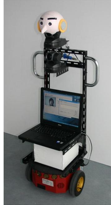
Fig. 4. Guide robot. The robot consists of a mobile robot, Pioneer II by ActivMedia, a laptop PC, and two pan-tilt-zoom cameras.
